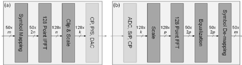
**Fig. 1** (a): Transmitter design. (b): Receiver design. (CP: cyclic prefix, P/S: parallel-to-serial, S/P: serial-to-parallel.) The dark grey boxes are included in synthesized ASIC designs, while the light grey boxes are used in simulation only.
